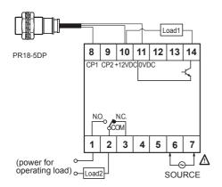
The sum of operating current capacity of load 1 and sensor should not be over external power capacity (50mA).
