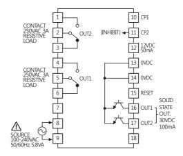
XINHIBIT: In case of timer mode, this terminal is for time hold. (voltage input (PNP): connect with 12VDC, no-voltage input (NPN): connect with 0VDC)
