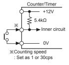
**%CP1**, CP2 (INHIBIT), RESET input part
