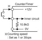
**%CP1**, CP2 (INHIBIT), RESET input part
