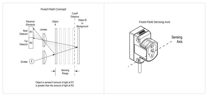
In the drawings and information provided in this document, the letters E, R1, and R2 identify how the sensor's three optical elements (Emitter "E", Near Detector "R1", and Far Detector "R2") line up across the face of the sensor. The location of these elements defines the sensing axis, see "Figure: Fixed-Field Sensing Axis" on page 2.
