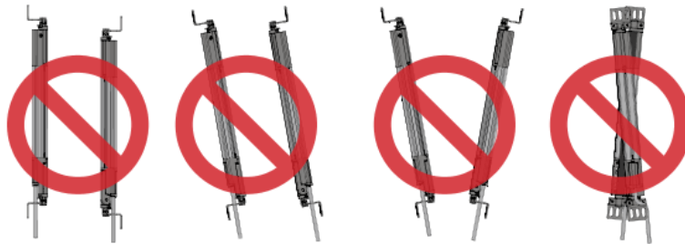
Figure 14. Incorrect Sensor Alignment
