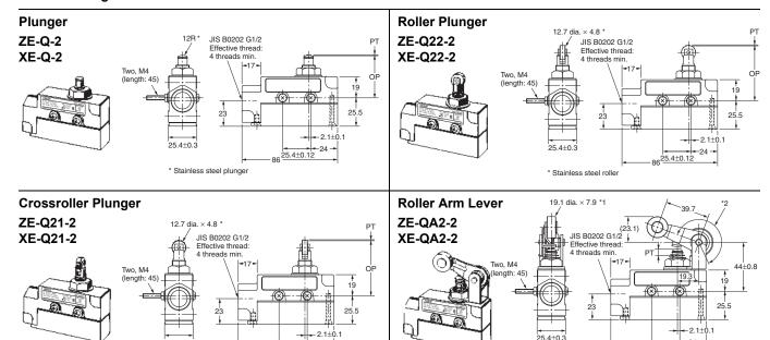
Note: 1. Unless otherwise specified, a tolerance of  $\pm 0.4$  mm applies to all dimensions
