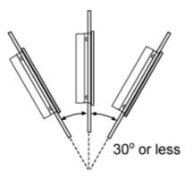
When installing the panel in a slanted position with an incline more than  $30^{\circ}$ , the ambient temperature must not exceed 40 °C (104 °F). You may need to use forced air cooling (fan,A/C) to ensure the ambient operating temperature is  $40^{\circ}$ C or less (104 °F or less).
