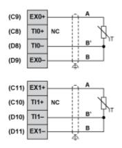
2 Wiring for Analog Inputs PT100
