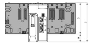
a: additional space below the rack to accommodate the height of the CPU. For an X Bus rack, the value is 30.9 mm (1.217 in.); for an Ethernet rack, the value is 29.49 mm (1.161 in.).
