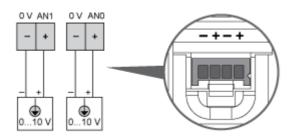
The (-) poles are connected internally.
