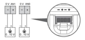
The (-) poles are connected internally.
