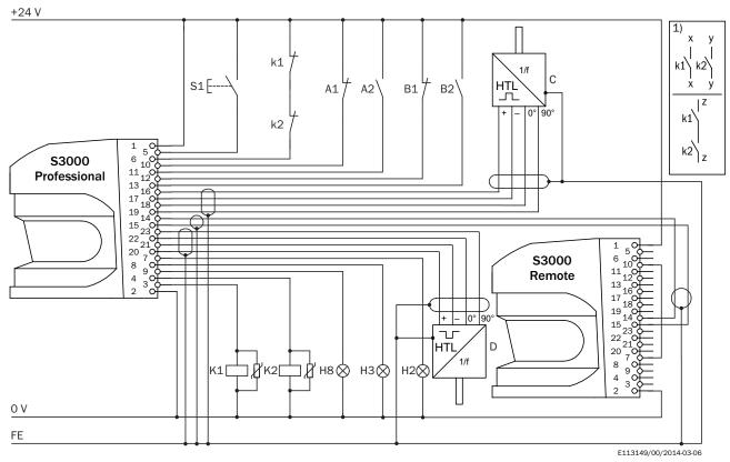
S3000 Professional (left) and Remote (right) in conjunction with relays/contactors
