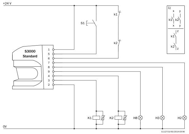
S3000 Standard in conjunction with relays/contactors
