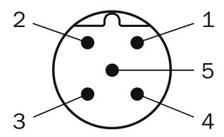
Male connector M12, 5-pin, A-coded
