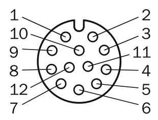
M12, 12-pin female connector, A-coded (I/O)
