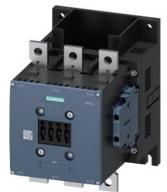
power contactor, AC-3e/AC-3 300 A, 160 kW / 400 V, without operating mechanism 3-pole, auxiliary contacts 2 NO + 2 NC main circuit: busbar control and auxiliary circuit: screw terminal
