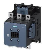
power contactor, AC-3e/AC-3 300 A, 160 kW / 400 V, AC (50-60 Hz) / DC Uc: 96-127 V PLC input 24 V DC 3-pole, auxiliary contacts 2 NO + 2 NC drive: electronic main circuit: busbar control and auxiliary circuit: screw terminal
