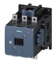
power contactor, AC-3e/AC-3 400 A, 200 kW / 400 V AC (50-60 Hz) / DC Uc: 200-277 V PLC input 24 V DC 3-pole, auxiliary contacts 2 NO + 2 NC drive: electronic main circuit: busbar control and auxiliary circuit: screw terminal
