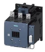
power contactor, AC-3e/AC-3 400 A, 200 kW / 400 V AC (50-60 Hz) / DC Uc: 200-277 V PLC input 24 V DC 3-pole, auxiliary contacts 1 NO + 1 NC drive: electronic main circuit: busbar control and auxiliary circuit: screw terminal with remaining lifetime indicator
