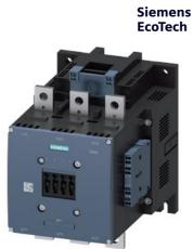
power contactor, AC-3e/AC-3 500 A, 250 kW / 400 V AC (50-60 Hz) / DC Uc: 440-480 V 3-pole, auxiliary contacts 2 NO + 2 NC drive: conventional main circuit: busbar control and auxiliary circuit: spring-loaded terminal
