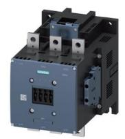
power contactor, AC-3e/AC-3 500 A, 250 kW / 400 V AC (50-60 Hz) / DC Uc: 21-27.3 V PLC input 24 V DC 3-pole, auxiliary contacts 2 NO + 2 NC drive: electronic main circuit: busbar control and auxiliary circuit: screw terminal
