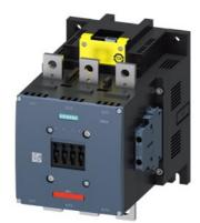
power contactor, AC-3e/AC-3 500 A, 250 kW / 400 V AC (50-60 Hz) / DC 96-127 V x (0.8-1.1) F-PLC input 24 V DC 3-pole, auxiliary contacts 2 NO + 2 NC permanently mounted drive: electronic main circuit: busbar control and auxiliary circuit: screw terminal
