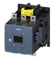
power contactor, AC-3e/AC-3 500 A, 250 kW / 400 V AC (50-60 Hz) / DC 96-127 V x (0.8-1.1) F-PLC input 24 V DC 3-pole, auxiliary contacts 2 NO + 2 NC drive: electronic main circuit: busbar control and auxiliary circuit: screw terminal
