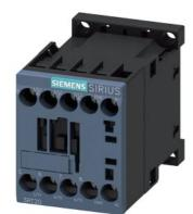
power contactor, AC-3e/AC-3, 7 A, 3 kW / 400 V, 3-pole, 24 V AC, 50/60 Hz, auxiliary contacts: 1 NC, screw terminal, size: S00, upright mounting position
