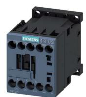
power contactor, AC-3e/AC-3, 7 A, 3 kW / 400 V, 3-pole, 400 V AC, 50 Hz / 400-440 V, 60 Hz, auxiliary contacts: 1 NO, screw terminal, size: S00
