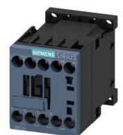
power contactor, AC-3e/AC-3, 7 A, 3 kW / 400 V, 3-pole, 480 V AC, 60 Hz, auxiliary contacts: 1 NC, screw terminal, size: S00
