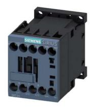
power contactor, AC-3e/AC-3, 7 A, 3 kW / 400 V, 3-pole, 24 V DC, auxiliary contacts: 1 NC, screw terminal, size: S00, upright mounting position
