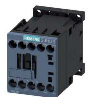
power contactor, AC-3e/AC-3, 7 A, 3 kW / 400 V, 3-pole, 125 V DC, auxiliary contacts: 1 NO, screw terminal, size: S00
