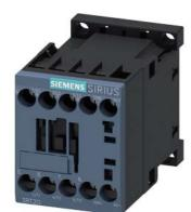
power contactor, AC-3e/AC-3, 7 A, 3 kW / 400 V, 3-pole, 48 V DC, auxiliary contacts: 1 NC, screw terminal, size: S00  $\,$
