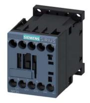
power contactor, AC-3e/AC-3, 7 A, 3 kW / 400 V, 3-pole, 24 V DC, with integrated varistor, auxiliary contacts: 1 NC, screw terminal, size: S00  $\,$
