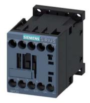
power contactor, AC-3e/AC-3, 7 A, 3 kW / 400 V, 3-pole, 24 V DC, 0.85-1.85\* Us, with integrated diode, auxiliary contacts: 1 NC, screw terminal, size: S00, not expandable with auxiliary switch
