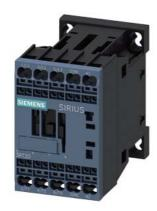
power contactor, AC-3e/AC-3, 7 A, 3 kW / 400 V, 3-pole, 24 V AC, 50/60 Hz, auxiliary contacts: 1 NC, spring-loaded terminal, size: S00
