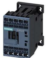
power contactor, AC-3e/AC-3, 9 A, 4 kW / 400 V, 3-pole, 110 V AC, 50/60 Hz, auxiliary contacts: 1 NO, spring-loaded terminal, size: S00  $\,$
