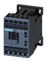
power contactor, AC-3e/AC-3, 9 A, 4 kW / 400 V, 3-pole, 230 V AC, 50/60 Hz, auxiliary contacts: 1 NC, spring-loaded terminal, size: S00  $\,$
