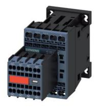
power contactor, AC-3e/AC-3, 9 A, 4 kW / 400 V, 3-pole, 230 V AC, 50/60 Hz, auxiliary contacts: 2 NO + 2 NC, spring-loaded terminal, size: S00, captive auxiliary switch
