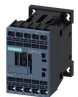
power contactor, AC-3e/AC-3, 9 A, 4 kW / 400 V, 3-pole, 220 V AC, 50 Hz / 240 V, 60 Hz, auxiliary contacts: 1 NO, spring-loaded terminal, size: S00
