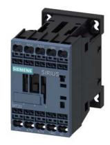
power contactor, AC-3e/AC-3, 9 A, 4 kW / 400 V, 3-pole, 400 V AC, 50/60 Hz, auxiliary contacts: 1 NO, spring-loaded terminal, size: S00  $\,$
