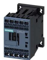
power contactor, AC-3e/AC-3, 9 A, 4 kW / 400 V, 3-pole, 24 V DC, auxiliary contacts: 1 NO, spring-loaded terminal, size: S00, upright mounting position
