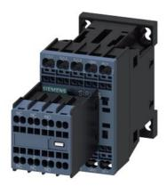
power contactor, AC-3e/AC-3, 9 A, 4 kW / 400 V, 3-pole, 24 V DC, auxiliary contacts: 2 NO + 2 NC, spring-loaded terminal, size: S00, removable auxiliary switch
