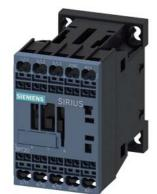
power contactor, AC-3e/AC-3, 9 A, 4 kW / 400 V, 3-pole, 60 V DC, auxiliary contacts: 1 NC, spring-loaded terminal, size: S00  $\,$
