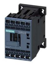
power contactor, AC-3e/AC-3, 9 A, 4 kW / 400 V, 3-pole, 110 V DC, auxiliary contacts: 1 NC, spring-loaded terminal, size: S00  $\,$
