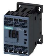
power contactor, AC-3e/AC-3, 9 A, 4 kW / 400 V, 3-pole, 125 V DC, auxiliary contacts: 1 NC, spring-loaded terminal, size: S00  $\,$
