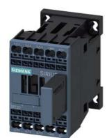
power contactor, AC-3e/AC-3, 9 A, 4 kW / 400 V, 3-pole, 24 V DC, with varistor plugged on, auxiliary contacts: 1 NO, spring-loaded terminal, size: S00, upright mounting position
