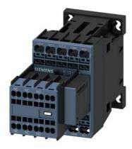
power contactor, AC-3e/AC-3, 9 A, 4 kW / 400 V, 3-pole, 24 V DC, with varistor plugged on, auxiliary contacts: 2 NO + 2 NC, spring-loaded terminal, size: S00, removable auxiliary switch
