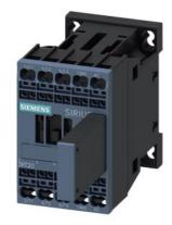
power contactor, AC-3e/AC-3, 9 A, 4 kW / 400 V, 3-pole, 230 V AC, 50/60 Hz, with plugged-on RC element, auxiliary contacts: 1 NO, spring-loaded terminal, size: S00
