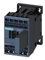
power contactor, AC-3e/AC-3, 9 A, 4 kW / 400 V, 3-pole, 230 V AC, 50/60 Hz, with plugged-on RC element, auxiliary contacts: 1 NC, spring-loaded terminal, size: S00
