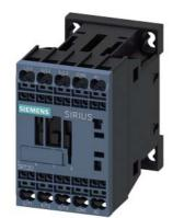
power contactor, AC-3e/AC-3, 9 A, 4 kW / 400 V, 3-pole, 110 V AC, 50/60 Hz, with integrated full-wave rectifier, auxiliary contacts: 1 NC, spring-loaded terminal, size: S00
