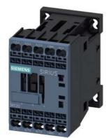
power contactor, AC-3e/AC-3, 9 A, 4 kW / 400 V, 3-pole, 24 V DC, 0.7-1.25\* Us, with integrated diode, auxiliary contacts: 1 NO, spring-loaded terminal, size: S00, suitable for PLC outputs, not expandable with auxiliary switch
