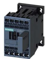
power contactor, AC-3e/AC-3, 9 A, 4 kW / 400 V, 3-pole, 24 V DC, 0.7-1.25\* Us, with varistor plugged on, auxiliary contacts: 1 NO, spring-loaded terminal, size: S00, not expandable with auxiliary switch
