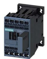
power contactor, AC-3e/AC-3, 9 A, 4 kW / 400 V, 3-pole, 24 V DC, 0.7-1.25\* Us, with varistor plugged on, auxiliary contacts: 1 NC, spring-loaded terminal, size: S00, not expandable with auxiliary switch
