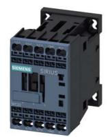
power contactor, AC-3e/AC-3, 9 A, 4 kW / 400 V, 3-pole, 24 V DC, 0.85-1.85\* Us, with integrated suppressor diode, auxiliary contacts: 1 NO, spring-loaded terminal, size: S00
