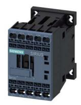
power contactor, AC-3e/AC-3, 9 A, 4 kW / 400 V, 3-pole, 24 V DC,  $0.85-1.85^{*}$  Us, with integrated suppressor diode, auxiliary contacts: 1 NC, spring-loaded terminal, size: S00
