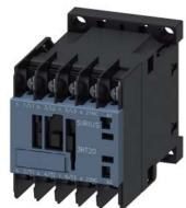
power contactor, AC-3e/AC-3, 9 A, 4 kW / 400 V, 3-pole, 100 V AC, 50 Hz / 100-110 V, 60 Hz, auxiliary contacts: 1 NC, ring cable lug connection, size: S00  $\,$
